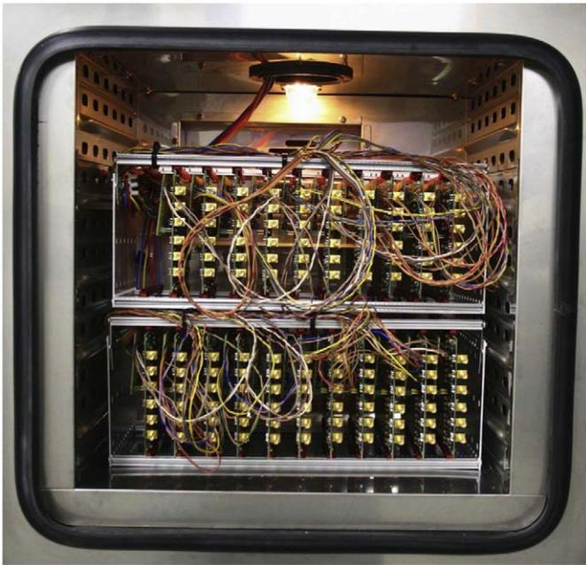
**Fig. 3.** Up to 22 FEBs were placed in a climate chamber for burn-in under electric power.
