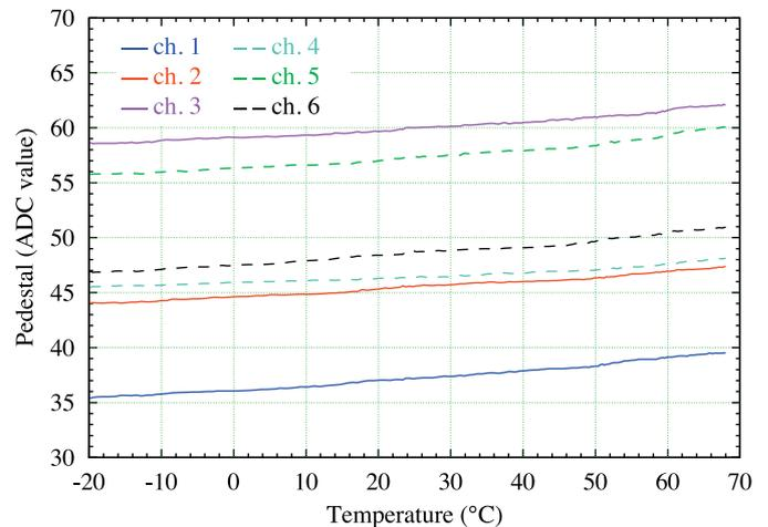
Fig. 7. Pedestals (in ADC-counts) for the six channels of an individual FEB as a function of temperature.
