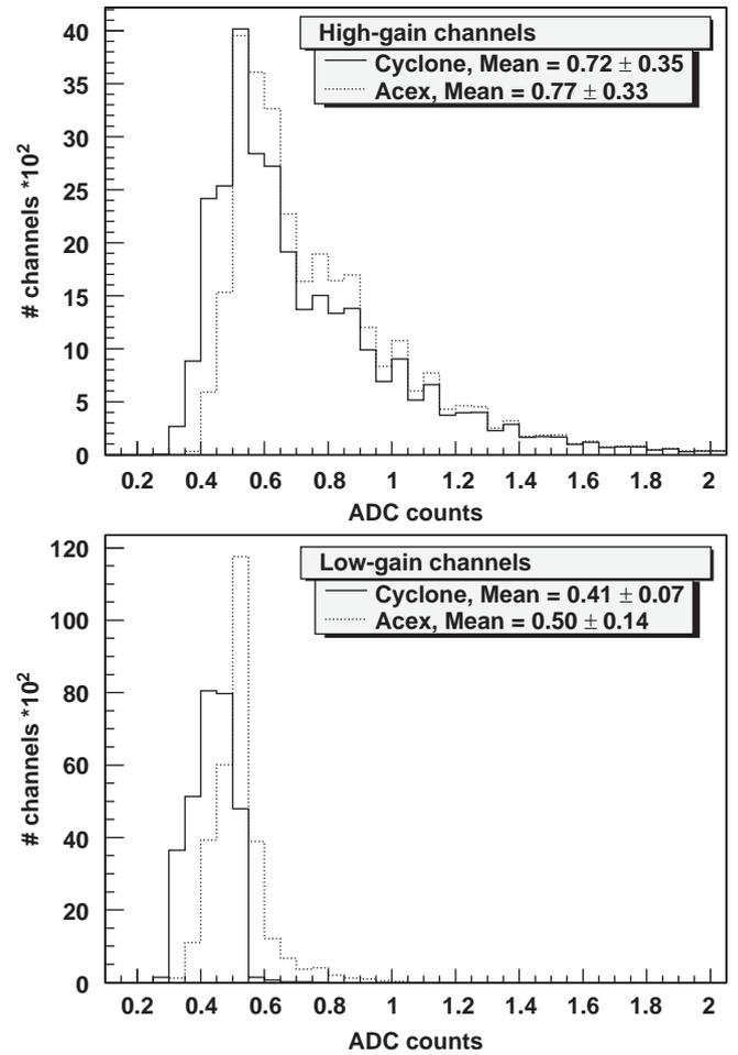
Fig. 9. Comparison of the noise levels for the high- (top) and low-gain channel (bottom) for the Cyclone and ACEX FEBS measured in April 2008, for 175 386 events registered in Cyclone FEBS and 324 035 events registered in ACEX FEBS. In field conditions  $\sigma_{Cyclone}^{high-gain} = 0.72$ , while  $\sigma_{ACEX}^{high-gain} = 0.77$  and  $\sigma_{Cyclone}^{low-gain} = 0.41$ , while  $\sigma_{ACEX}^{low-gain} = 0.50$ . The graphs are normalized to the amount of events.
