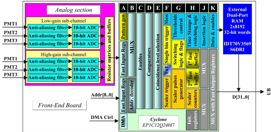
**Fig. 1.** Structure of the Front-End Board. Three high-gain and three low-gain channels amplify and shape the analog signals from three PMTs (anode and dynode) in 5-pole Bessel anti-aliasing filters. The shaped signals are digitized in six ADCs and further processing is performed in the Cyclone™ FPGA. All processes are split into sub-processes performed in the single clock cycle and encapsulated in the A,B,C,... procedures.
