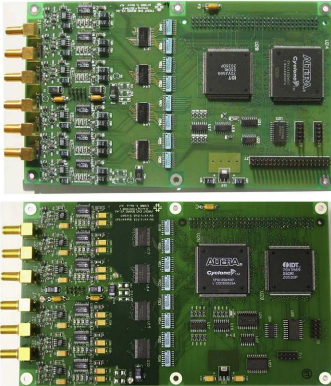
**Fig. 2.** The Cyclone™ 3rd generation prototype (top) and production (bottom) Front-End Board.
