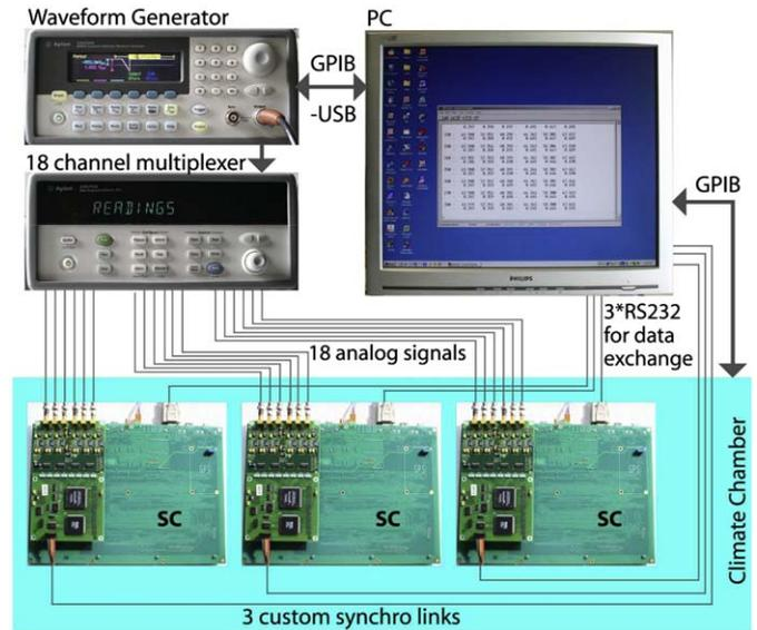
**Fig. 5.** Sketch of the automated test system.
