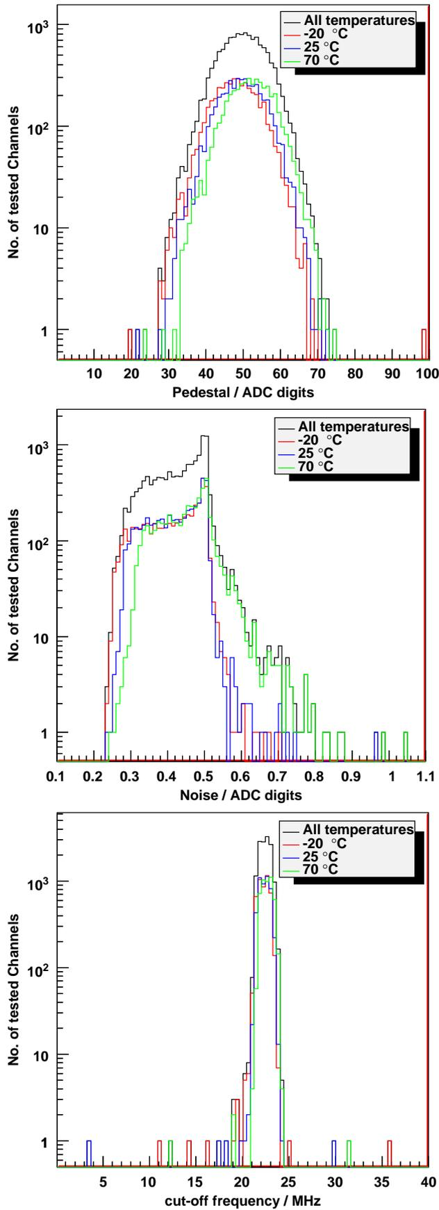
Fig. 8. Pedestals, noise and cut-off frequencies vs. temperature as measured in the lab.
