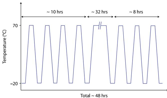
**Fig. 4.** The temperature profile for the “burn-in” test.
