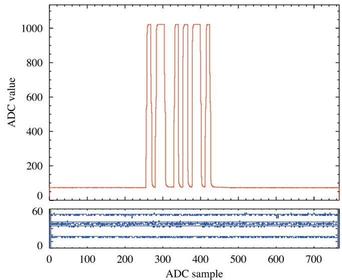
Fig. 10. A test pulse driving a reference channel. The oscillation from the pedestal up to the saturation is constrained between the 256th and the 429th time bin (with 25 ns grid) (above). No crosstalk is observed (bottom). The neighboring channels are running with the floating, not connected inputs.
