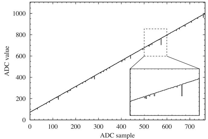
Fig. 6. Artificial non-linearity due to a jitter of data outgoing from the FADC.
