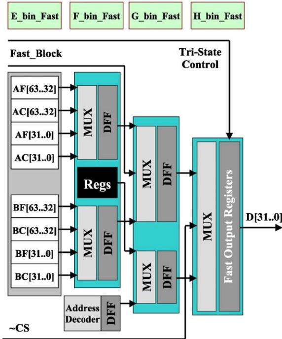
Fig. 7. The structure of the pipeline readout system.
