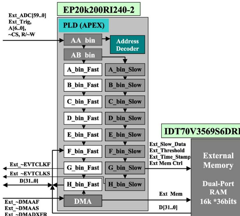
Fig. 6. Pipeline structure of the internal routines.
