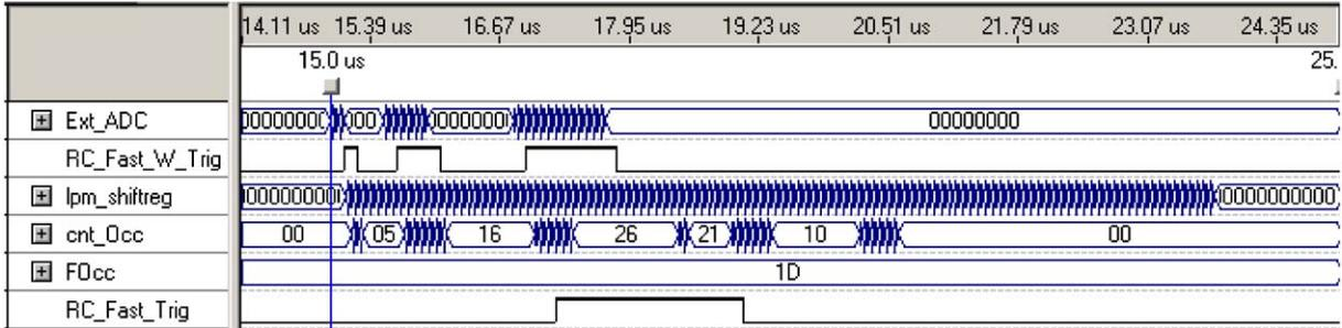
Fig. 3. An example of time-over-threshold trigger simulation. Three input pulses (signal Ext\_ADC) generate preliminary triggers (RC\_Fast\_W\_Trig) which propagate in the shift register (lpm\_shiftreg). The final trigger (RC\_Fast\_Trig) is generated when the occupancy (cnt\_Occ) is above the required value (FOcc).
